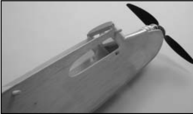
B. Install dowels and place a drop of medium CA to hold dowels in
