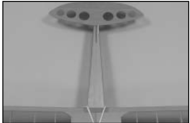
B. Determine the top and bottom of the stab like this: the sealed edge of the elevator should be on top, and the beveled edge be on the bottom.
