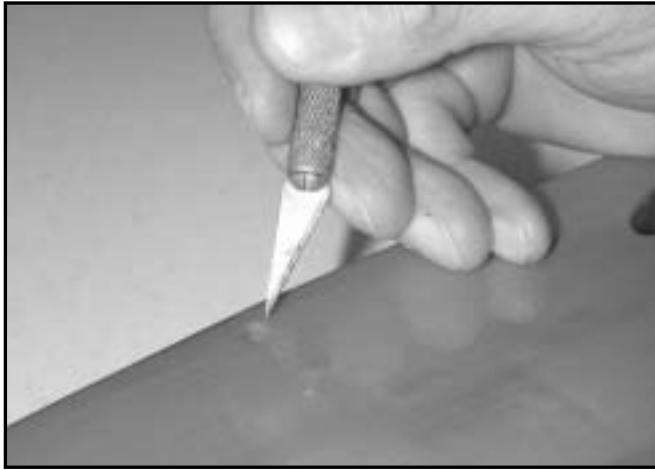
A. Cut away the covering film from the predrilled holes in the fuselage with a hobby knife.
